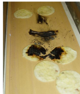
Field Strength Effect Very close slices in very high field intensity lead to arcing
