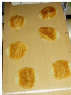
Field Vector Effect Left-Right edges were not heated at all, even when centre of chip was scorched
