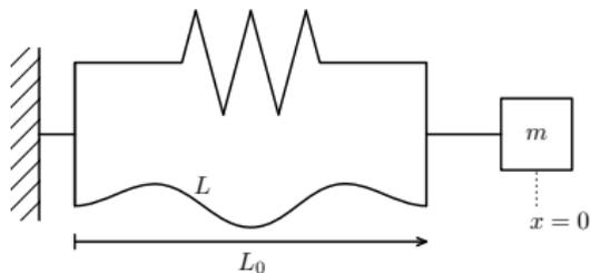
**Figure:** A mass-spring-wire system in its equilibrium
