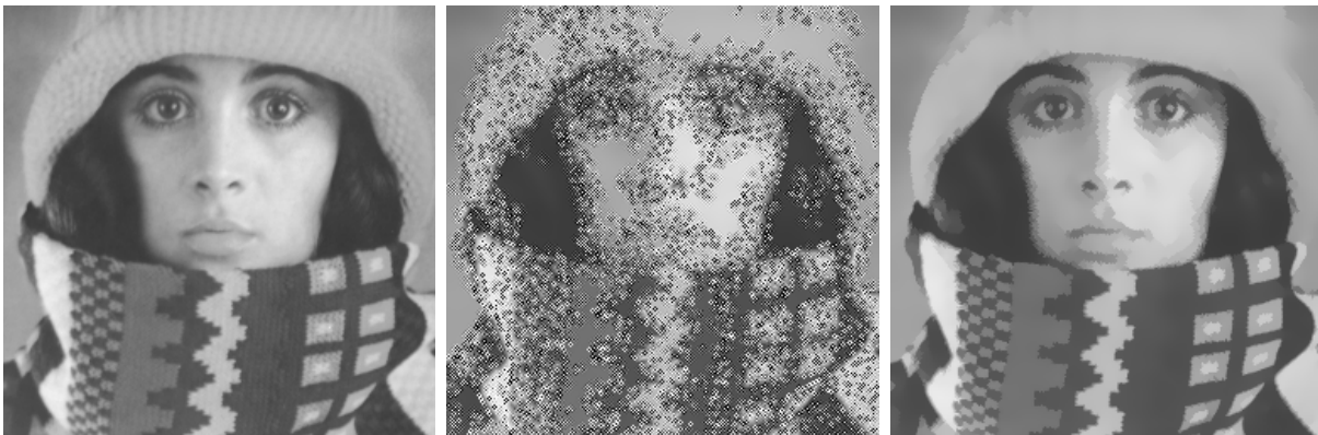
(a) Left: Original image, 256 \times 256 pixels. (b) Middle: After filtering with an explicit scheme for FAB diffusion with Bogdan diffusivity ( \lambda_1 = 4 , \lambda_2 = 10 ) and standard discretisation (100 iterations with \tau = 0.1 ). (c) Right: Same with nonstandard discretisation.
